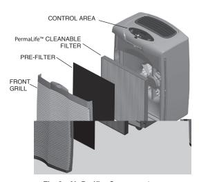
Fig. 2 - Air Purifier Components
